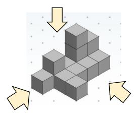
**Step 2:** Sketch the plan with the correct scale. Label the sketch with 'plan elevation'.
