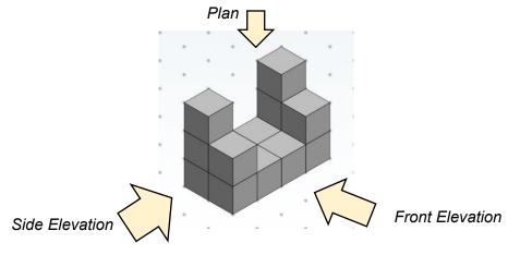
**Step 2:** Sketch the plan with the correct scale. Label the sketch with 'plan elevation'.
